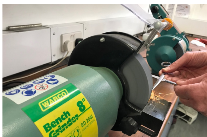
Figure 12: Repair of surgical scissors
