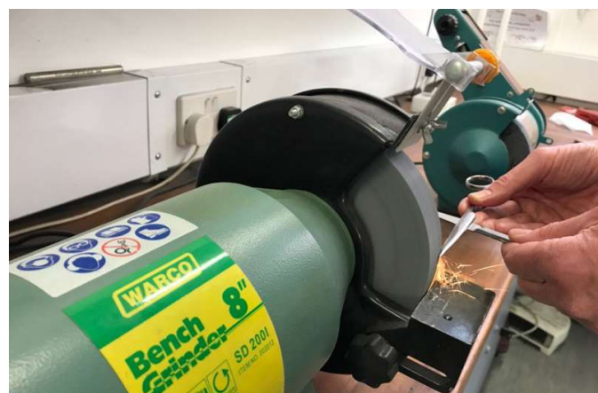
Figure 12: Repair of surgical scissors
